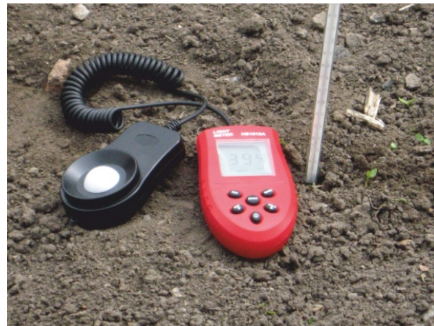
Fig.4. Instruments for measuring illumination and soil temperature
