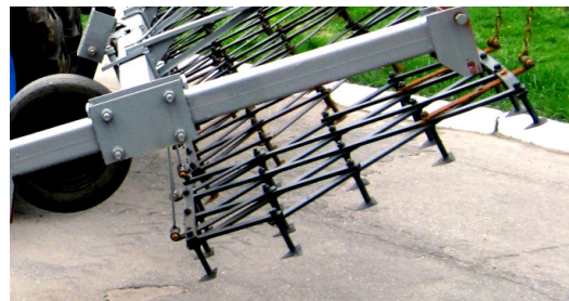
Fig. 2. Working bodies of the harrow for processing fallow, equipped with flat cutting teeth
